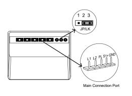
Lock Control Jumper: To select the lock type.
